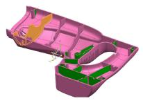
product design and identify key features such as bends, embossing and sheet metal thickness that influence the manufacturing of stamping tools. Once the features are analyzed and identified, the information is transferred to Teamcenter tool costing software to estimate manufacturing costs.
